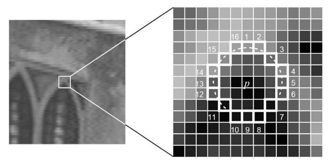
12-POINT SEGMENT TEST: CORNER DETECTION IN AN IMAGE PATCH.
