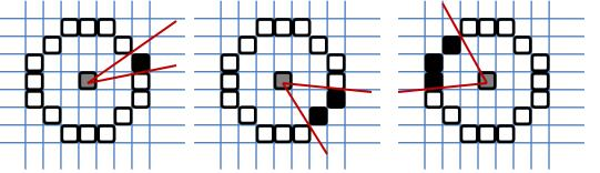
In digital space, corner is defined as a neighborhood of radius 3 where N consecutive pixels are all brighter than the center pixel by at least the threshold TO and the remaining 16-N consecutive pixels are darker than the bright pixels by at least the threshold T. For sharp corners, N = 13, 14, 15 (usually, 14 and 15). This test is for dark objects on light background. There is a similar test for bright objects on dark background.
